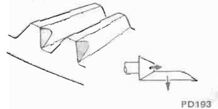
Fig. PD-28 Heel contact
