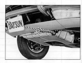
Fig. GI-11 Front towing point
